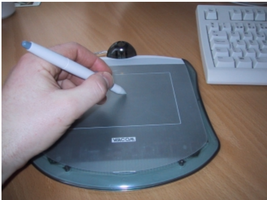
Fig. 3: Natural writing on digitizer tablet in order to control virtual drawing pointer.
