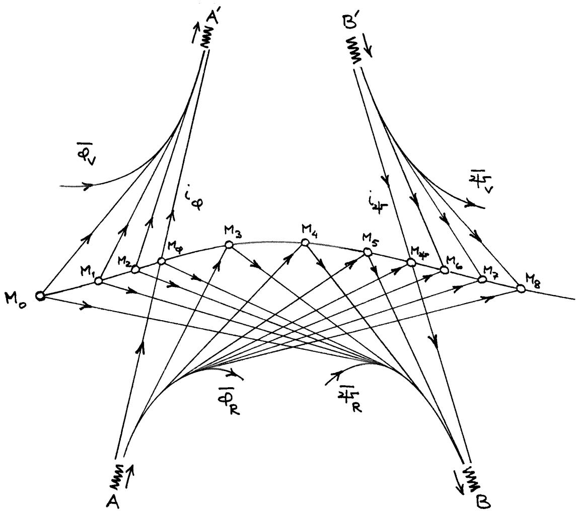
Suppose we are given two caustics  $\bar{\phi}$  and  $\bar{\phi}^*$  as in figure , each consisting of two arcs with a common asymptotic ray  $i_{\bar{\phi}}$  and  $i_{\bar{\phi}^*}$  respectively. Localizing the mirror as in the figure (choosing  $M_0$  and finding the rays of  $\bar{\phi}$  and  $\bar{\phi}^*$  that intersect at  $M_0$ ) gives us a real and a virtual arc of each caustic ( $\bar{\phi}_R$  and  $\bar{\phi}_V$  real,  $\bar{\phi}_V$  and  $\bar{\phi}_R^*$  virtual ).
