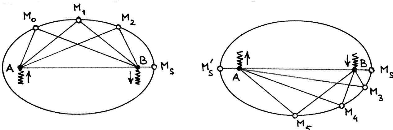
Starting at  $M_0$ , letting out string from A and pulling it in at B, the pen will move through  $M_1, M_2, \dots$  tracing out the desired ellipse until it reaches the vertex-point  $M_s$  at the end of the major axis.
