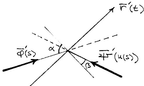
$$(6) \quad \begin{cases} \langle \bar{\varphi}'(s), \bar{r}'(t) \rangle = |\bar{r}'(t)| \cos(\frac{\pi}{2} - \alpha) = |\bar{r}'(t)| \sin \alpha \\ \langle \bar{r}'(u(s)), \bar{r}'(t) \rangle = |\bar{r}'(t)| \cos(\frac{\pi}{2} + \beta) = -|\bar{r}'(t)| \sin \beta \end{cases}$$
