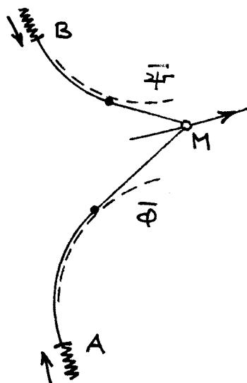
AS THE PEN MOVES, IT WILL TRACE OUT THE LOCALLY HYPERBOLIC MIRROR THAT REFLECTS THE REAL (VIRTUAL)  $\bar{\phi}$  INTO THE VIRTUAL (REAL)  $\bar{\tau}\bar{r}$  AND PASSES THROUGH THE STARTING POINT OF THE PEN
