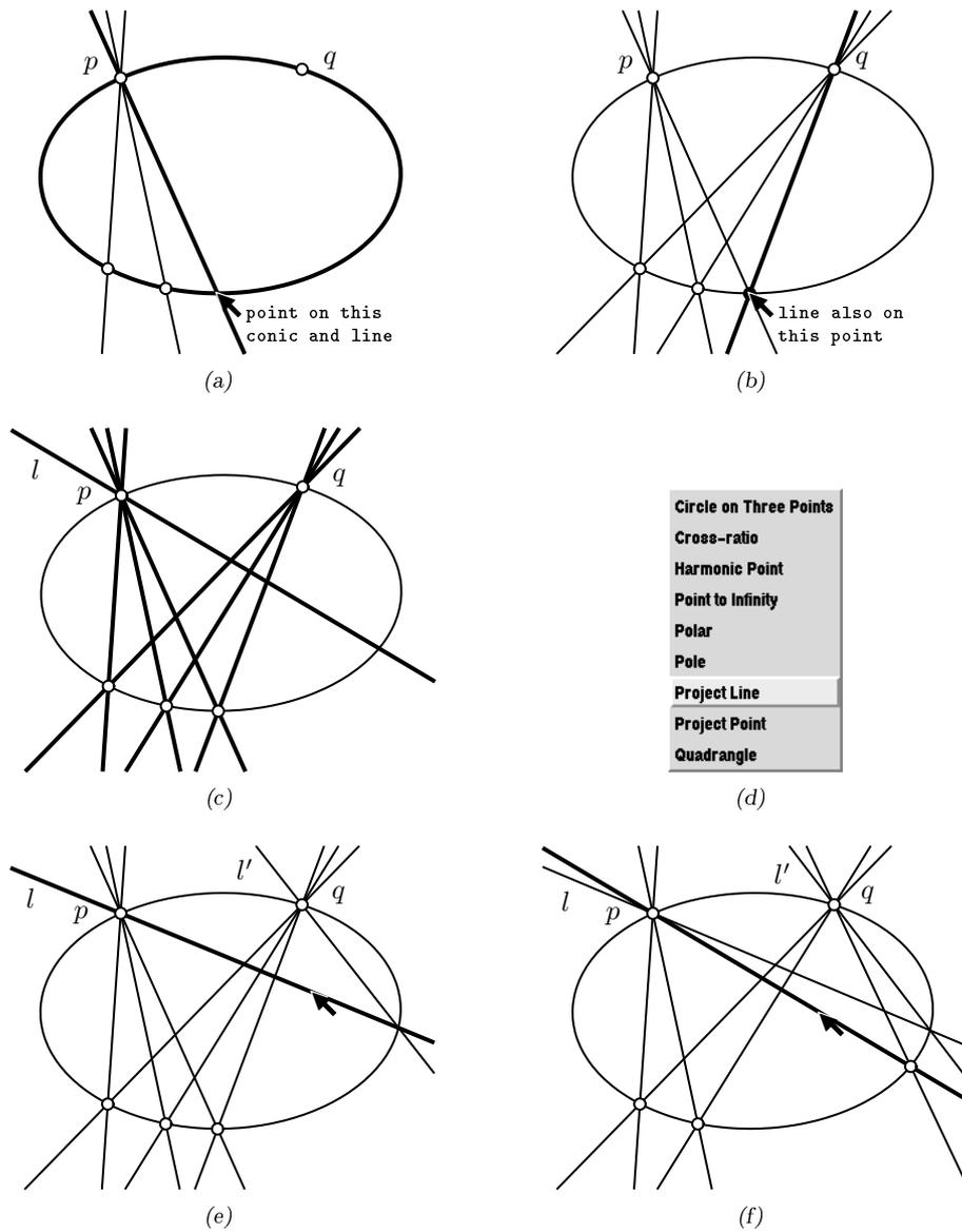
Figure 6.14. Constructing the projectivity which defines the conic.
