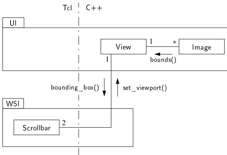
Figure 5.72. If the View sends bounding box information directly to the scrollbar, the View has to know the Tcl name of the scrollbar, which makes the View dependent on Tcl.
