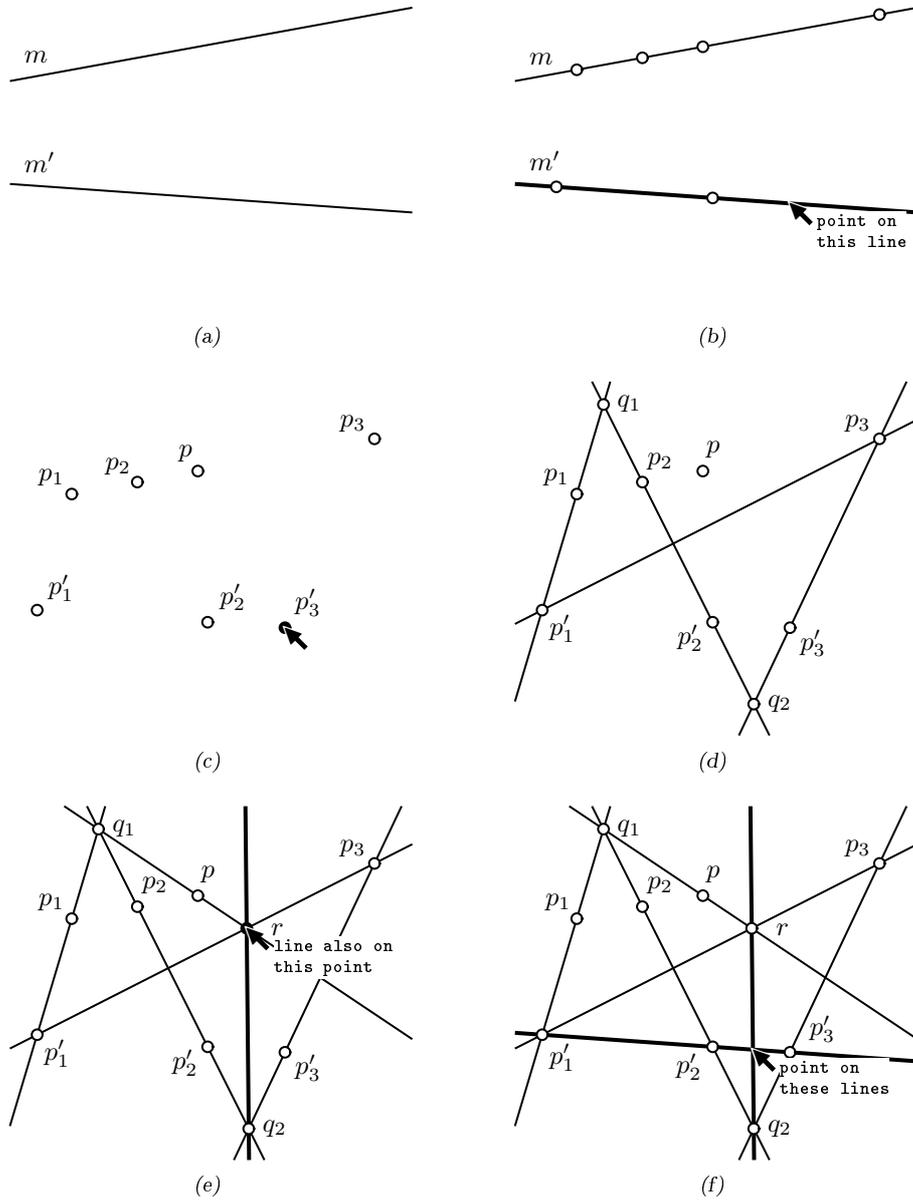
Figure 6.13. Constructing the  $P_1$  projectivity which maps three collinear points to three other collinear points.
