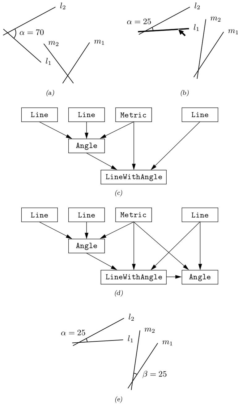
Figure 5.32. The orientation of  $m_2$  is constrained by the angle between  $l_1$  and  $l_2$ .
