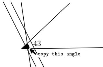
Figure 5.50. If the measurement tool is active, the lines obscuring the angle symbol will be ignored which makes it easy to select the angle.
