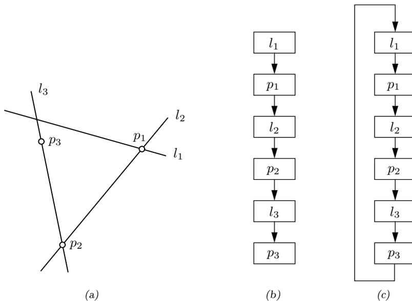
Figure 5.43. If the user were allowed to attach  $l_1$  to  $p_3$ , a cycle would be created in the dependency graph.
