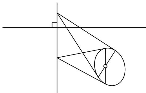
Figure 1.3. A perspective view of a tire in a vertical plane. The optical axis of the camera is parallel to the ground plane.
