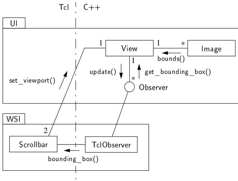
Figure 5.73. If the `View` instead uses an abstract `Observer` interface, all Tcl-dependent code can be collected into a `TclObserver` class which implements the `Observer` interface. The `TclObserver` is responsible both for fetching the current bounding box from the `View` when `update` is called, and for passing that information on to the scrollbars.
