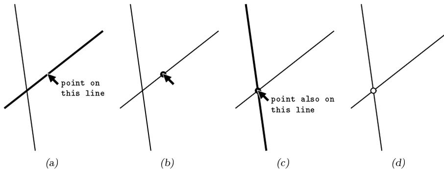
Figure 5.39. Another constraint can be added before the mouse button is released.
