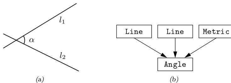
Figure 5.31. Measuring the angle between two lines.
