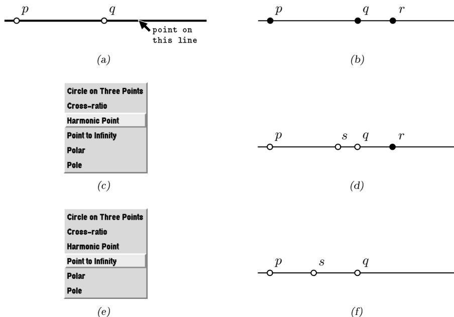
Figure 6.16. Constructing the midpoint of a line segment  $pq$ .
