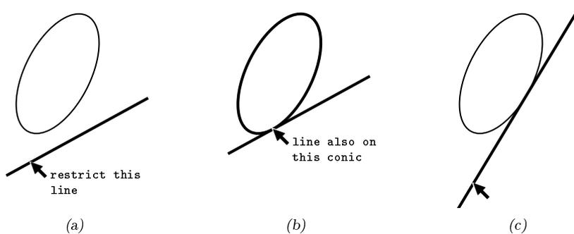
Figure 5.40. Constraints can be added to existing objects.
