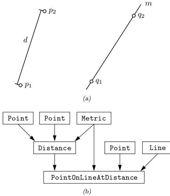
Figure 5.36. A constraint has been put on  $q_2$  so that the distance  $q_1q_2$  equals the distance  $p_1p_2$ .
